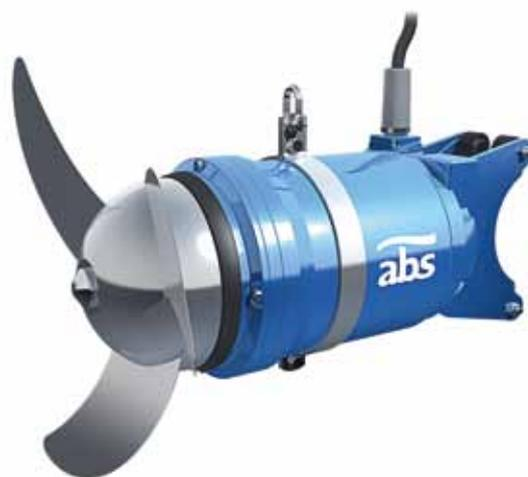
The ABS submersible mixer XRW has a permanent-magnet motor IE3 equivalent to achieve the lowest energy consumption possible for medium-speed mixing. Up to 35% energy can be saved compared with other existing medium-speed mixer designs.
